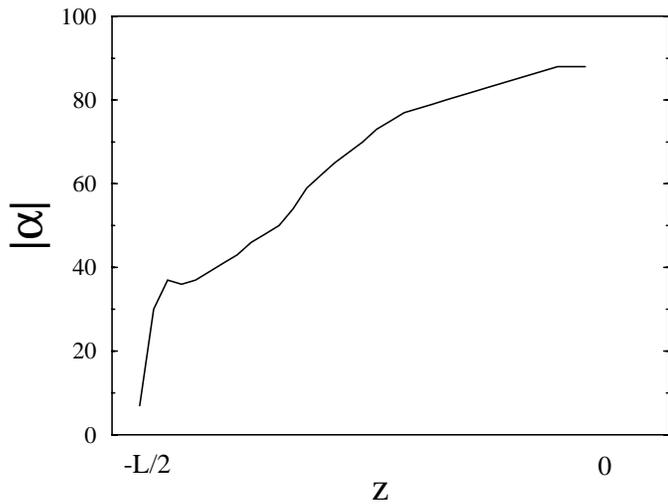
**Fig. 7.** The maximum value of  $\alpha$  is plotted as a function of the axial coordinate  $z$ , obtained for  $\nu = \eta = 5.62 \cdot 10^{-5}$ .
