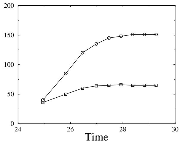
**Fig. 5.** Resistive time evolution (for  $\eta = \nu = 10^{-4}$ ) of maximum values of current density amplitude (square) and azimuthal velocity (circle), measured at the loop apex. The values are reported in arbitrary units in order to be plotted on the same graph.
