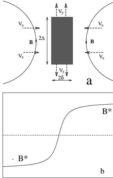
**Fig. 1a and b.** Schematic representation of the reconnection process. Intense gradients in the magnetic field are formed by compression due to plasma flow in the  $x$  direction **b**. The reconnection layer (shaded area) where diffusive effect is dominant represents a two dimensional region of extent  $2\delta * 2\Delta$  **a**.
