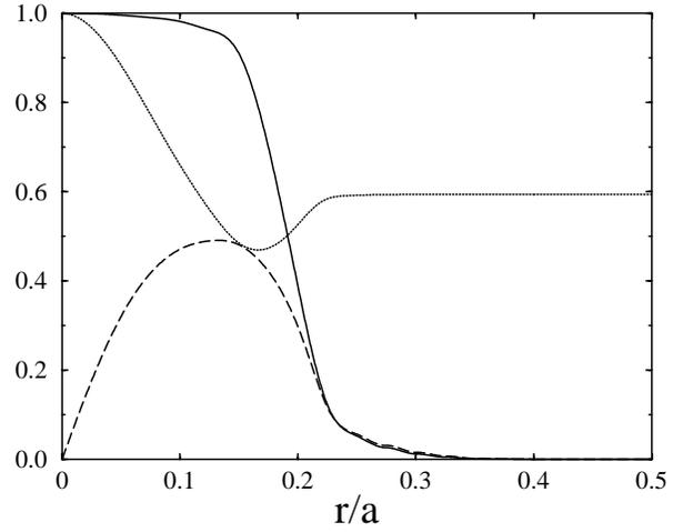
**Fig. 2.** The twist profile  $\Phi(r)$  (plain line) and the corresponding azimuthal  $B_\phi$  (dashed line) and axial  $B_z$  (dotted line) components of the equilibrium magnetic field. The magnetic field and twist values are normalized to their values on the magnetic axis.
