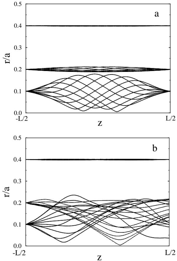
**Fig. 3a and b.** Mapping of three sets of ten field lines originating from  $r/a = 0.1, 0.2,$  and  $0.4$  at  $z = -L/2$ , projected into the  $(r, z)$  plane, at the end of the ideal phase **a** and at a given time during the resistive phase **b**.
