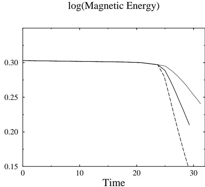
**Fig. 4.** Time evolution of the azimuthal magnetic energy for three dissipation coefficient values,  $\eta = \nu = \sqrt{10} \cdot 10^{-4}$  (dashed line),  $10^{-4}$  (plain line), and  $\sqrt{10} \cdot 10^{-5}$  (dotted line).
