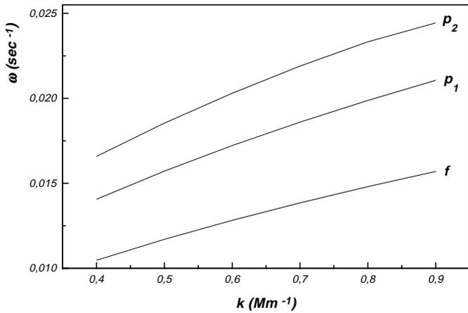
Fig. 2. The diagnostic diagram for the shell without magnetic field
