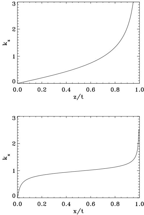
**Fig. 2.** Vertical (upper panel) and horizontal (lower panel) distributions of wavenumbers as a function of  $z/t$  or  $x/t$ , where  $t$  is fixed and  $x, z \leq t$ .
