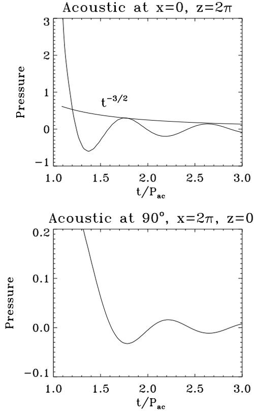
**Fig. 10.** Pressure amplitude of the wake (in arbitrary units) vs time at  $x = 0$  and  $z = 2\pi$  (top panel) and at  $x = 2\pi$  and  $z = 0$ . The pulse has been removed; the amplitude decay of  $t^{-3/2}$  is given as a comparison in the top panel.
