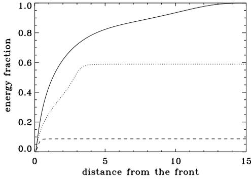
**Fig. 11.** The fractional energy contained inside a cone vs distance from the front, for a cone whose axis is inclined at  $0^\circ$  (—),  $45^\circ$  (· · ·), and  $90^\circ$  (- - -) with respect to the vertical.
