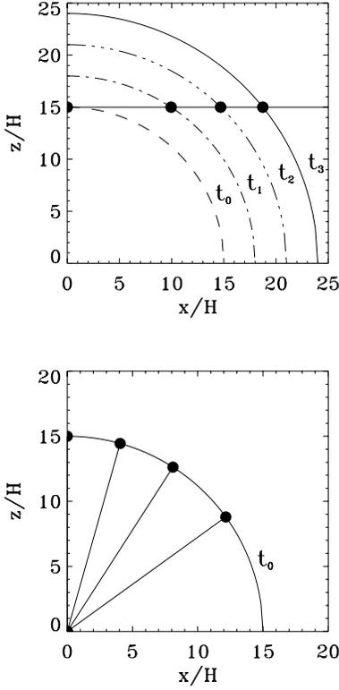
**Fig. 7.** Upper panel represents the positions of a wave crest at different times and their intersections with height of  $15H$ . Lower panel shows a wave crest whose apex has reached the height of  $15H$  at time  $t_0$ .
