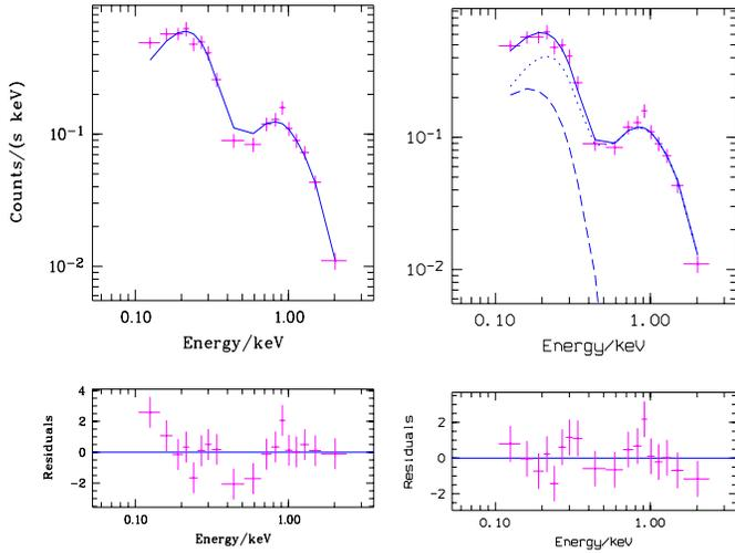
**Fig. 2.** X-ray spectrum (pointed obs.) of RX J0134-4258 and residuals. *Left:* The upper panel gives the observed X-ray spectrum (crosses) and powerlaw model fit (solid line), the lower panel the residuals. *Right:* The same for a powerlaw plus black body fit (the quality of the fit is improved, but some systematic residuals around 0.4-0.9 keV remain). The spectrum was binned to a signal/noise of  $8\sigma$  per bin. The amount of cold absorption was fixed to the Galactic value.
