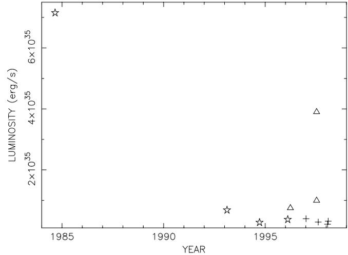
**Fig. 6.** Luminosity history of RX J0146.9+6121. The luminosities are in the 2–10 keV band and for a distance of 2.5 kpc. Triangles and crosses refer to *RossixTE* and *BeppoSAX* observations respectively while stars to data collected by other satellites (EXOSAT, ROSAT and ASCA). Except for the 1984 and July 1997 outbursts, all the flux measurements are consistent with an average luminosity of  $\sim 5 \times 10^{34}$  erg s $^{-1}$ .
