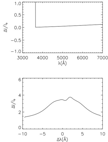
**Fig. 3.** Continuum emission and  $H\alpha$  line profile generated by a condensation ( $P_0=30$ ,  $\Delta Z=14$  km, and  $T=9240$  K) in an atmosphere represented by the model F2.
