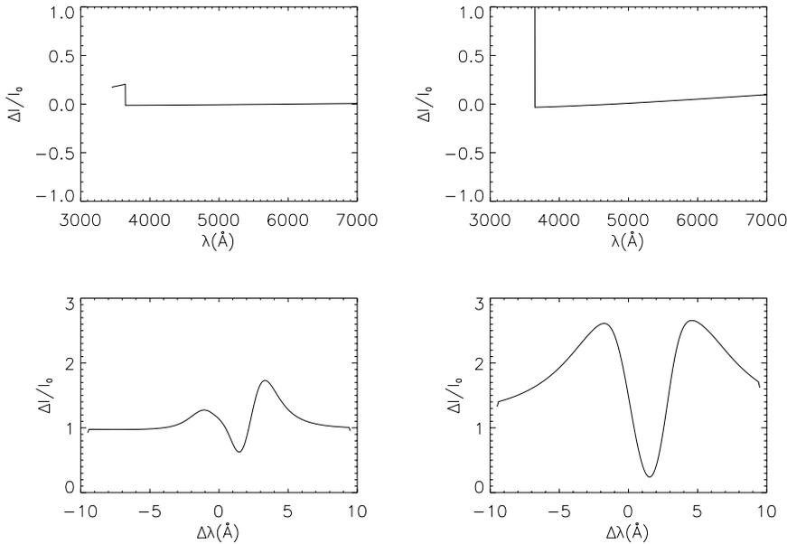
**Fig. 4.** In an atmosphere represented by the model G2, continuum emission and  $H\alpha$  line profile generated by a chromospheric condensation ( $P_0=100$ ,  $\Delta Z=80$  km, and  $T=10600$  K) alone (left panel) or complemented by non-thermal effects with  $F_{20}=10^{11}$  ergs  $\text{cm}^{-2}\text{s}^{-1}$  and  $\delta=3$  (right panel).
