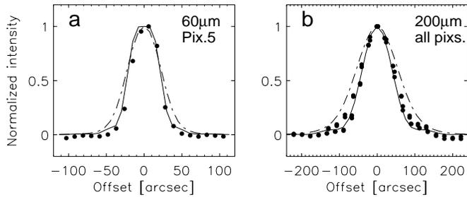
**Fig. A.1.** Comparison of measured and modelled footprints of ISOPHOT. The intensity profiles (dots) were measured along the satellite Y-direction. Dash-dot lines mark the modelled footprint of extended sources with  $\text{FWHM}=30''$  at  $60\mu\text{m}$  and  $\text{FWHM}=60''$  at  $200\mu\text{m}$
