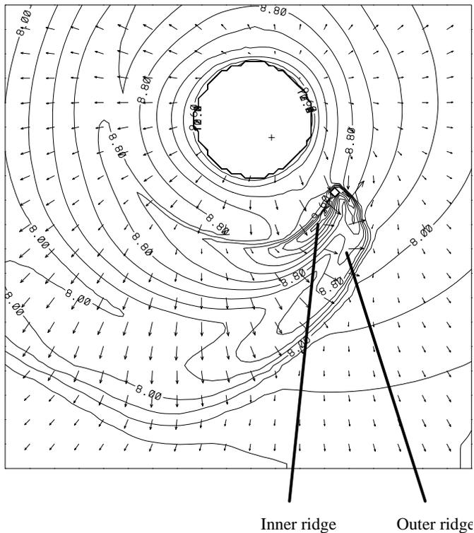
**Fig. 4.** Hydrodynamical simulation for the RW Hya system. Density (logarithmic) and projected velocity distribution in the orbital plane. Densities are given by contour lines, velocities by arrows. In the upper panel arrows of 1 mm correspond to a velocity of  $20 \text{ km s}^{-1}$ . The system rotates anti-clockwise. The center of mass is marked with a cross, The accretor is marked with a small circle.
