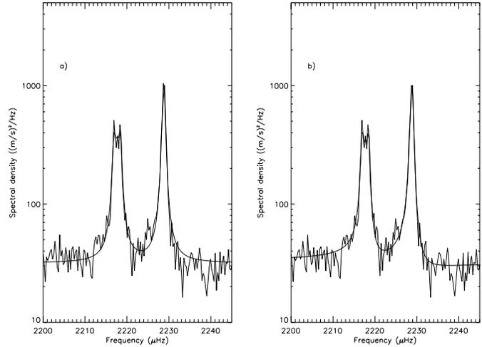
**Fig. 1a and b.** Example of fitting (modes  $\ell=0, n=15$  and  $\ell=2, n=14$ ) using Lorentzian profiles **a** and Nigam profiles **b**. Note the improved agreement (visible in the wings) between the fit and data when the asymmetry is taken into account. The resolution for the plot is reduced to  $0.29 \mu\text{Hz}$ .
