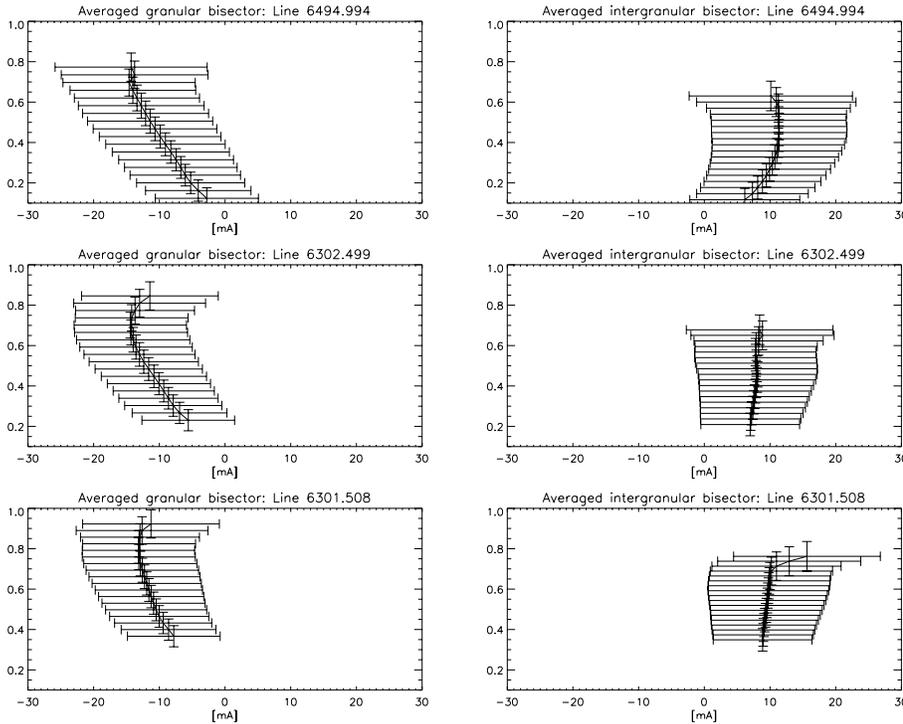
**Fig. 3.** Averaged granular and intergranular bisectors for spectrum nr. 162. In the case of the largest line core formation height the largest asymmetries result.
