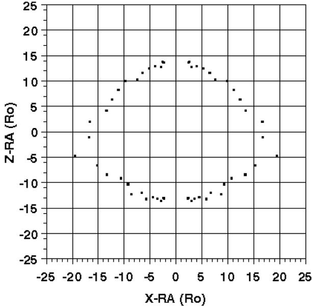
**Fig. 2.** The shape of the Alfvén surface based on measurements of Ulysses spacecraft during its first pole to pole journey.
