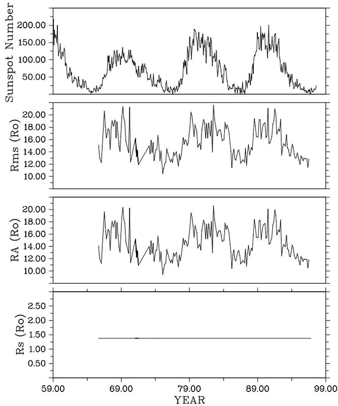
**Fig. 4.** Temporal variation of transition radii ( $R_s$ : sonic,  $R_A$ : Alfvén and  $R_{ms}$ : magnetosonic) based on in-ecliptic measurements at 1 AU. The sunspot number is presented as an index of solar activity.
