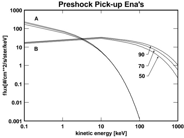
**Fig. 3.** Shown are preshock pick-up H-ENA spectra as function of energy in keV for various distances of the termination shock, i.e. for  $R_s = 50, 70, 90$  AU. Curves A are for normal turbulence levels, curves B for enhanced turbulence levels.
