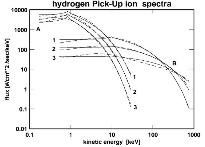
**Fig. 1.** Shown are calculated (dashed) and fitted (full) spectra of  $\text{H}^+$  pick-up ions as function of energy in keV for various distances: 1:  $R = 15$  AU; 2:  $R = 35$  AU; 3:  $R = 89$  AU. Curves A are for normal turbulence levels, curves B for enhanced turbulence levels.
