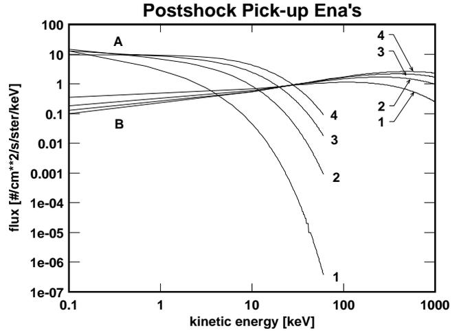
**Fig. 4.** Shown are postshock pick-up H-ENA spectra as function of energy in keV for various compression ratios  $s$  at the shock, i.e.  $s = 1, 2, 3, 4$ . Curves A are for normal turbulence levels, curves B for enhanced turbulence levels.
