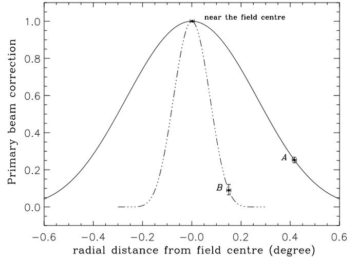
**Fig. 3.** Primary beam correction for the a typical WSRT antenna at 1.4 (—) and 5 GHz (---). A is an object 25' away from the 1.4-GHz pointing centre, and B is an object 9' away from the 5-GHz pointing centre. A small pointing error will not affect the flux density of objects near the centre of the field but will give a large error on the correction factor for an object near the edge of the primary beam.
