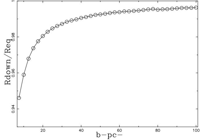
**Fig. 2.** The ratio  $R_{down}/R_{eq}$  versus  $b$  (in pc) when we have a linear decay of the density. The number of vertices along which we solve the differential equation is 2601,  $t_{final}=1.0 \cdot 10^4$  years,  $\Delta t = 1.0 \cdot 10^{-3} \cdot 10^4$  years,  $a=0.15$  particles  $\text{cm}^{-3}$  and  $c_a=0.1$ .
