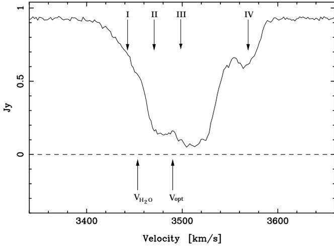
**Fig. 1.** Total neutral atomic hydrogen absorption averaged over the whole continuum. The upper arrows mark the velocity centroids of the four different spectral features (see Fig. 4). The two bottom arrows mark the optical systemic velocity and the velocity centroid of the systemic water maser features respectively
