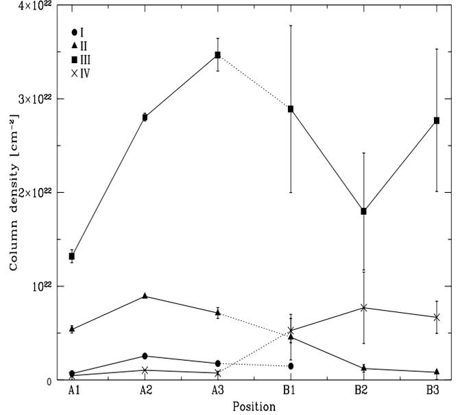
**Fig. 5.** The apparent H I column density distributions (assuming  $T_{\text{sp}} = 100 \text{ K}$  and a uniform covering factor) of the four spectral features (I-IV). Plotted is column density as a function of location across the VLBI source. The dotted lines represent an interpolation between the two continuum structures A and B. The errorbars are plotted at the one sigma level
