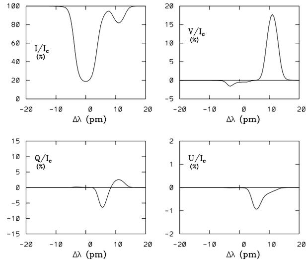
**Fig. 6.** Spatial averages of Stokes parameters of Fe I 5250.2 of 30 rays penetrating an embedded magnetic flux tube with 1500 G,  $30^\circ$ ,  $3 \text{ km s}^{-1}$  and tube width 0.5 in  $\log \tau_{c5}$ . The intersection depth of the rays with the upper surface of the flux tube varied linearly from  $-0.5$  to  $-4.5$  of  $\log \tau_{c5}$ . The Stokes  $V$  area asymmetry is  $-84 \%$  and the zero-crossing shift corresponds to  $2.3 \text{ km s}^{-1}$ .
