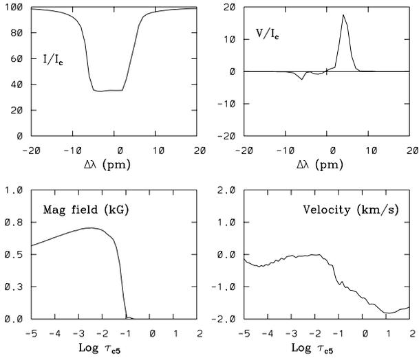
**Fig. 7.** Stokes  $I$  and Stokes  $V$  of Fe I 5250.2 of a ray penetrating the canopy area of a numerically simulated (non-stationary) magnetic flux slab at a chosen position and time (upper two panels). The lower two panels show magnetic field strength and velocity as function of  $\log \tau_{c5}$ . The area asymmetry of Stokes  $V$  is  $-75\%$ ; the value is negative because the velocity below the canopy is negative (up-flow).
