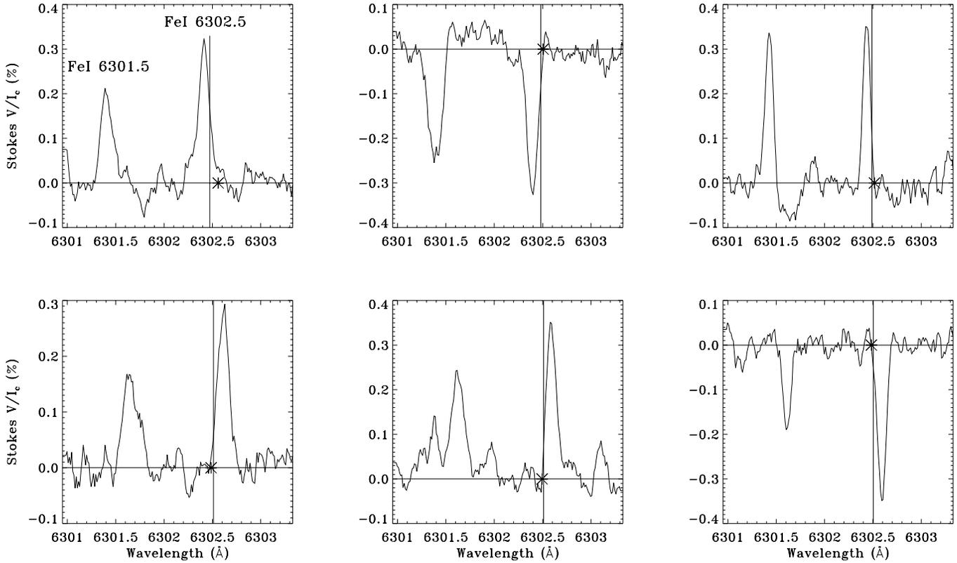
**Fig. 1.** Examples of observed one-lobe Stokes  $V$  profiles. Profiles with blue lobe only are shown in the upper, those with red lobe only in the lower row. Vertical solid lines mark the wavelength of the center of Stokes  $I$  and stars mark the Stokes  $V$  zero-crossing position (determined by extrapolation).
