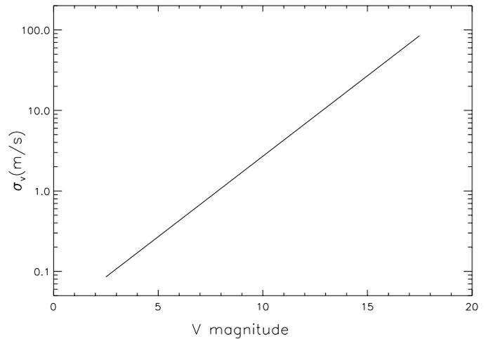
**Fig. 2.** Expected global error on the radial velocity as a function of the visible magnitude for a K7V star, observed during an equivalent integration time of 1 hour with the ELODIE spectrograph installed on the 2 m telescope of the OHP. The symbolic velocity error of  $1 \text{ ms}^{-1}$  is obtained for a visible magnitude 8 (see text).
