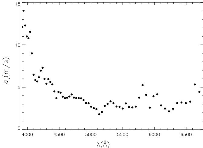
**Fig. 1.** Expected error on the radial velocity as a function of the wavelength (spectral order) for a K7V star of visible magnitude 6, observed during an equivalent integration time of 1 hour with the ELODIE spectrograph installed on the 2 m telescope of the OHP. Note that the main velocity information is contained beyond 4400 Å, where the error stabilizes around  $3 \text{ ms}^{-1}$  (see text).
