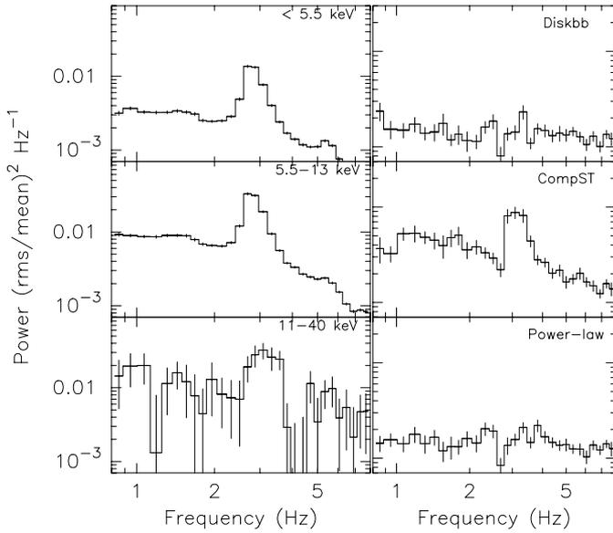
**Fig. 4.** The PDS in 3 energy ranges are shown in the left panels of the figure. In the right panels PDS generated after converting the light curves in 3 energy channels into light curves in three spectral components are shown.
