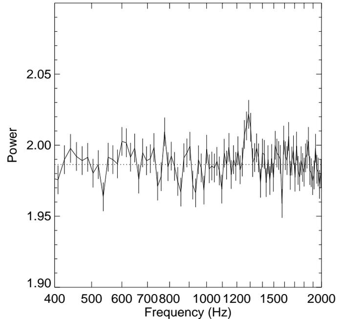
**Fig. 2.** Power spectrum for the 2460 s interval containing the QPO at  $1284 \pm 6$  Hz. The powers are Leahy normalized and have been rebinned for presentation. The dotted line shows the calculated Poisson noise level.
