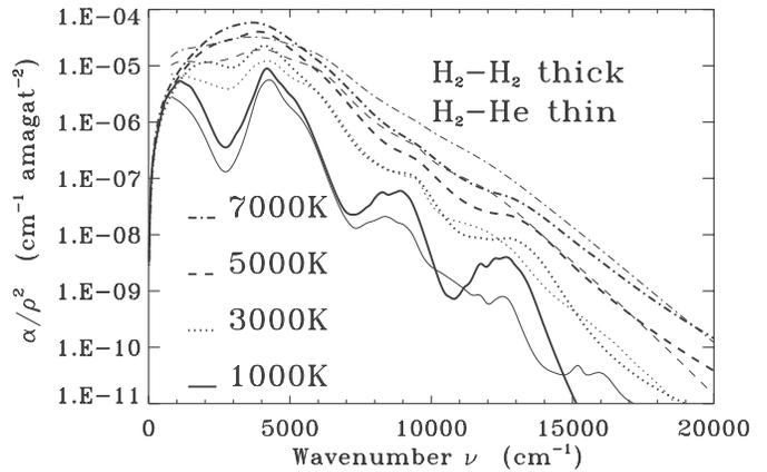
**Fig. 7.** Comparison of the most recent  $\text{H}_2$ - $\text{H}_2$  and  $\text{H}_2$ -He CIA absorption coefficients.
