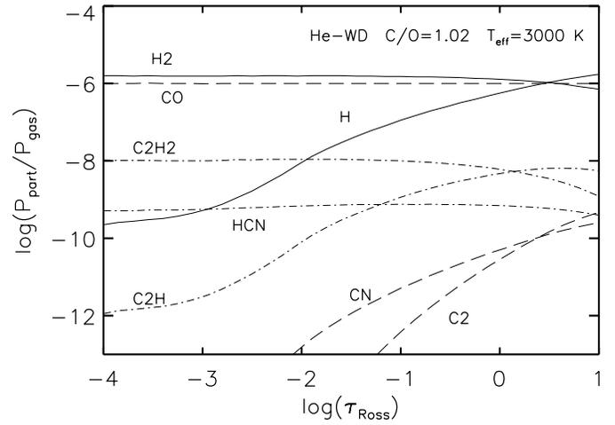
**Fig. 4.** The partial pressures of various molecules for the full opacity model atmosphere shown in Fig. 2. The partial pressures of H and  $\text{H}_2$  are shown as solid lines, diatomics (except  $\text{H}_2$ ) are shown as dashed lines, while polyatomics are shown by dash-dot lines. The names of the molecules are marked along the curves.
