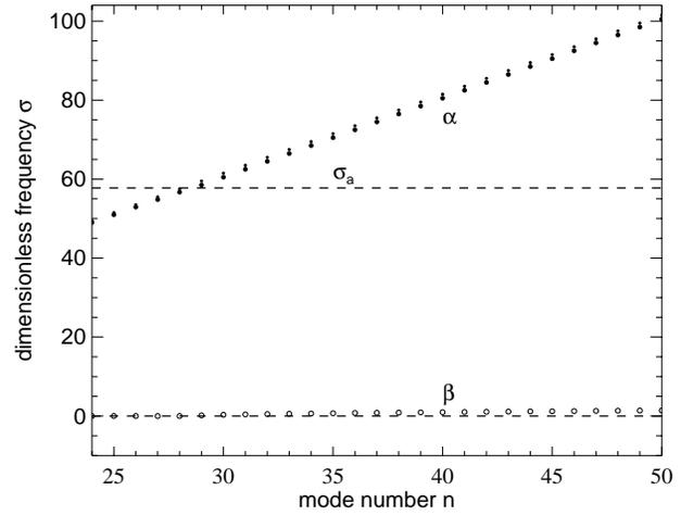
**Fig. 6.** Time damping coefficient  $\beta$  (open dots) and frequency  $\alpha$  (heavy solid dots) of quasi-stationary waves as functions of the order  $n$ . We have  $\sigma = \alpha + i\beta$ . The small dots indicate the real discrete frequencies of the atmosphere-free layer.
