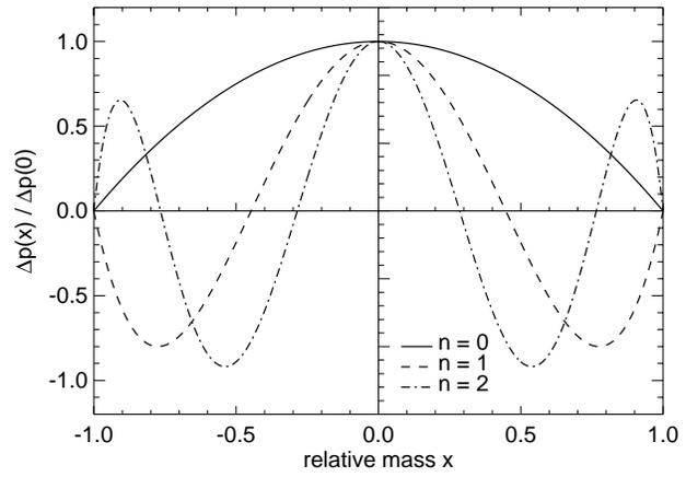
**Fig. 3.** The pressure perturbations of the three lowest normal modes as functions of the relative mass  $x$
