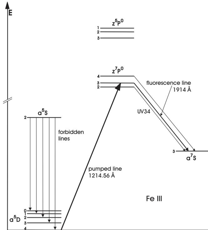
**Fig. 1.** Partial energy level diagram of Fe III, showing the energy levels involved in the forbidden lines and the fluorescent line discussed in the text. The energy axis is not to scale. Numbers beside the levels are J-values.
