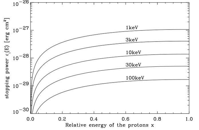
**Fig. 2.** Stopping power  $\varepsilon_I(E)$  vs. proton relative velocity  $x$  for different electron temperatures. The electron density is  $n_e = 10^{-19} \text{ cm}^{-3}$ .
