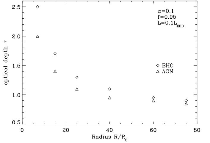
**Fig. 8.** Depth of the thermalization layer  $\tau_b$  as a function of distance from the central object for galactic BH case (diamonds) and AGN case (triangles). The thermalization depth is larger for the galactic black hole.
