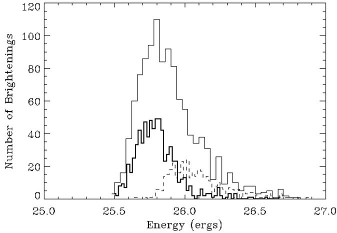
**Fig. 8.** The solid line shows the total energy, the thick line shows the cell energy and the dashed line shows the network energy.
