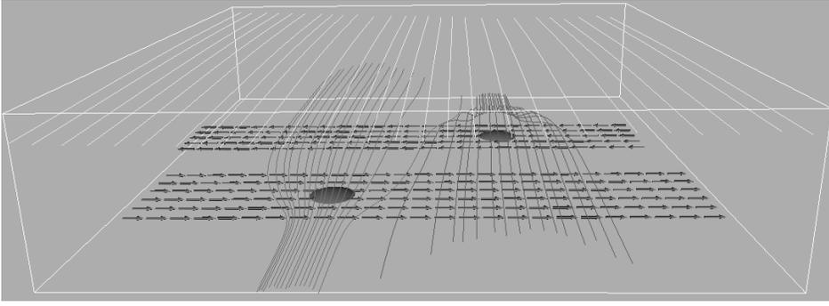
**Fig. 1.** The initial layout of the magnetic field topology. The isosurfaces indicate the locations of the two sources. The field lines indicate the locations of the magnetic separator surfaces that divides space into three independent flux regions and the overlaying open field. The vectors represent the topology of the imposed boundary driving.
