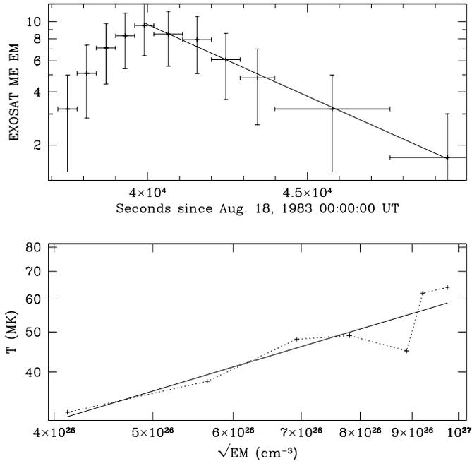
**Fig. 1.** The evolution of the EXOSAT Algol flare. The top panel shows the evolution of the emission measure during the flare, together with the best-fit exponential decay, while the bottom panel shows the evolution of the flare's decay in the  $\log T$  vs.  $\log n$  plane. The dotted line connects the points in their temporal order, while the solid line is the best fit to the decay.
