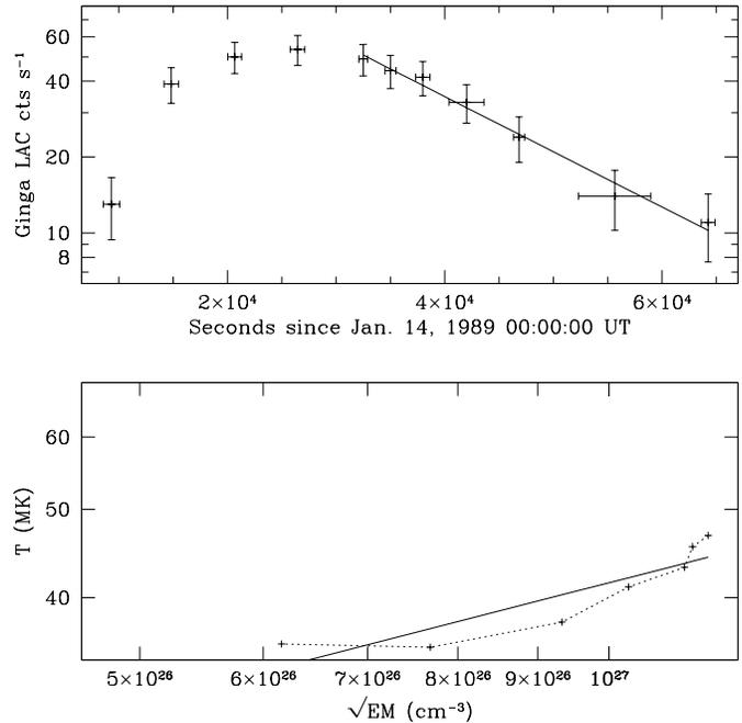
**Fig. 2.** The evolution of the GINGA Algol flare. The top panel shows the (background-subtracted) flare's light curve, together with the best-fit exponential decay, while the bottom panel shows the evolution of the flare's decay in the  $\log T$  vs.  $\log n$  plane. The dotted line connects the points in their temporal order, while the solid line is the best fit to the decay.
