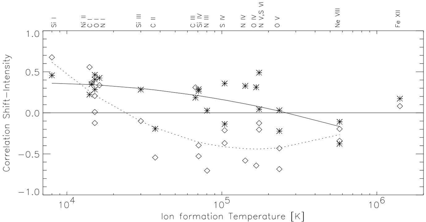
**Fig. 3.** Correlation coefficient between wavelength shifts and intensities, versus the ion formation temperatures. **Diamonds:** Coronal hole. **Stars:** Quiet Sun. The data are binned in intensity bins of 20 data points. The curves are quadratic fits to coronal hole (dashed) and quiet Sun (solid) data, not including the results of the Fe XII lines.
