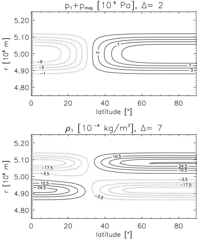
**Fig. 2.** Isolines of the total pressure perturbation ( $p_1 + p_{\text{mag}}$ ) and the density perturbation ( $\varrho_1$ ) for the same case as shown in Fig. 1. The magnetic curvature force is compensated by the latitudinal gradient of the total pressure perturbation. The hydrostatic equilibrium in the radial direction requires a density perturbation proportional to the radial gradient of the total pressure perturbation.
