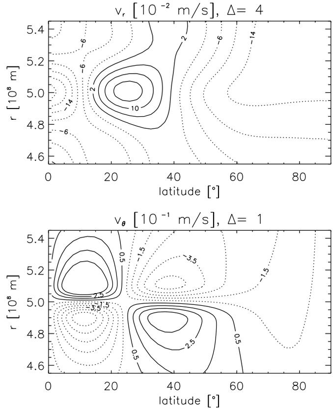
**Fig. 5.** Isolines of the meridional velocity field after  $5 \cdot 10^3$  s starting with the same magnetic field as in Fig. 4, but assuming initial force balance in the latitudinal direction. The unbalanced buoyancy force leads to an upflow in the region of strongest magnetic field around  $25^\circ$  latitude, whereas a downflow develops in the weak-field region near to the equator and the pole.
