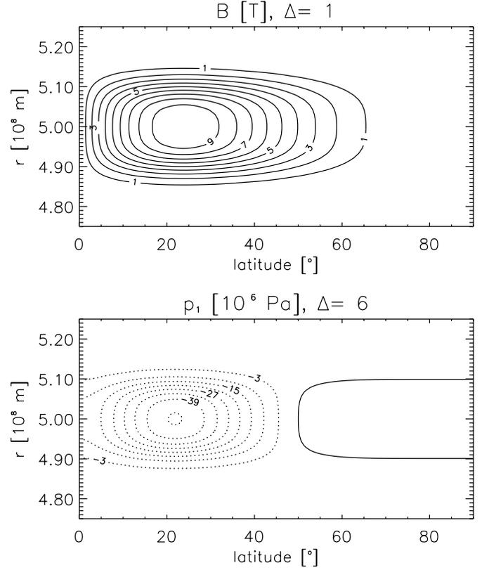
**Fig. 1.** Isolines of the magnetic field strength ( $B$ ) and the perturbation of the gas pressure ( $p_1$ ) for a magnetic layer without toroidal flow. The figures show a segment of the  $r - \theta$  plane, which is represented in a rectangular fashion for better visibility (latitude =  $90^\circ - \theta$ ). The symbol  $\Delta$  denotes the distance of the contour levels in the units given within the angular brackets.
