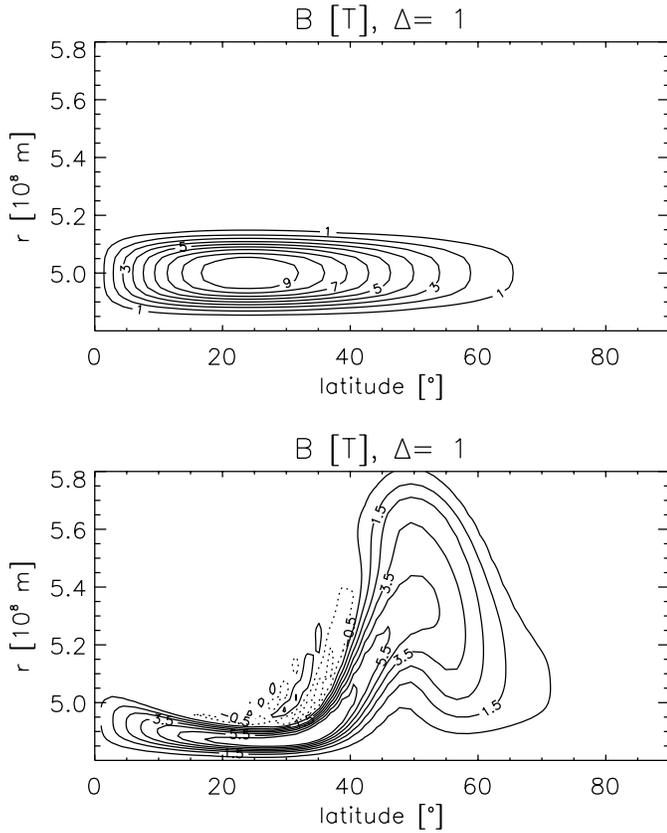
**Fig. 3.** Drift of a magnetic layer driven by an unbalanced magnetic curvature force in the absence of rotation. Upper panel: isolines of  $B$  for the initial state (same as in Fig. 1), lower panel: after 1 month simulated time. The simulation is performed with an adiabatic background stratification ( $\delta = 0$ ) and starting with force balance in radial direction.
