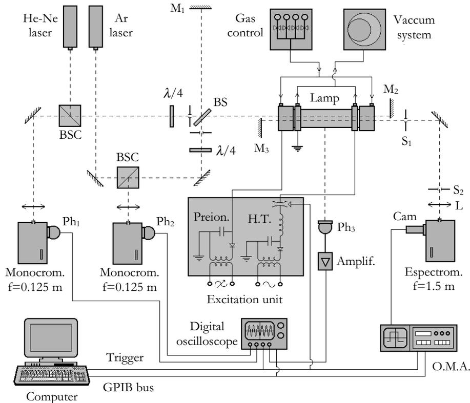
Fig. 1. Experimental arrangement.
