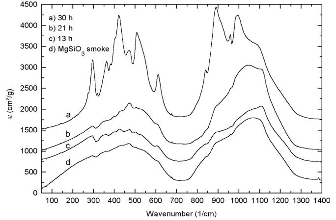
**Fig. 5.** Evolution of the MIR spectrum of  $\text{MgSiO}_3$  smoke after annealing at 1000 K up to 30 h. The annealing times are indicated. For clarity, the spectra are vertically shifted: a, b, c by  $+1500$ ,  $+1000$ ,  $+750\text{ cm}^2/\text{g}$ , respectively.
