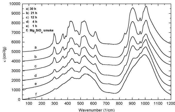
**Fig. 7.** Evolution of the MIR spectrum of  $\text{Mg}_2\text{SiO}_4$  smoke after annealing at 1000 K up to 30 h. The annealing times are indicated. For clarity, the spectra are vertically shifted: a, b, c, d, e by +5000, +4000, +3000, +2000, +1000  $\text{cm}^2/\text{g}$ , respectively.
