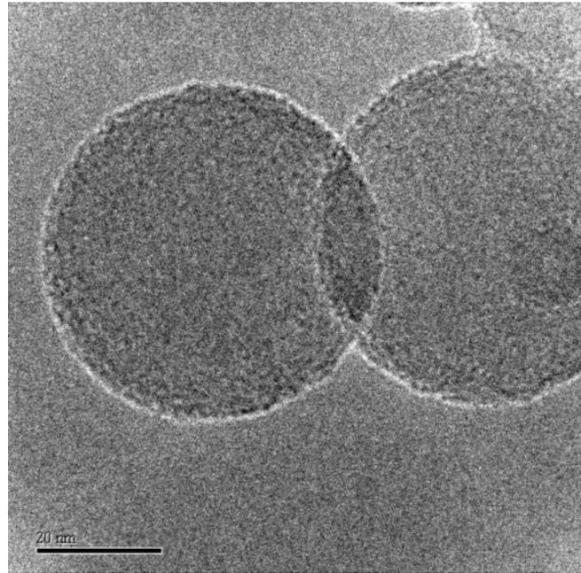
**Fig. 10.** TEM image of smaller-sized particles of the  $\text{Mg}_2\text{SiO}_4$  smoke after annealing up to 30 h at 1000 K. The Mg-poor particles that are characterized by a Mg/Si-ratio of about 1 seem to be structurally unchanged. However, they are partly crystalline as was checked by electron diffraction analyses.
