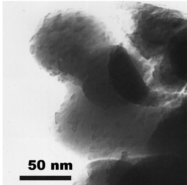
**Fig. 11.** TEM image of  $\text{Mg}_2\text{SiO}_4$  smoke that has been annealed at 1206 K for 1 h. Forsterite single crystals are embedded in a matrix made up of polycrystalline forsterite, crystalline and amorphous silica and MgO.
