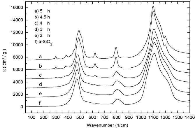
**Fig. 12.** Evolution of the MIR spectrum of silica that has been annealed at 1220 K. The annealing times are indicated. For clarity, the spectra have been shifted vertically: a, b, c, d, e by +7500, +6000, +4500, +3000, +2500 cm<sup>2</sup>/g, respectively.  $\tau$  has been approximated to 4.5 ± 0.5 h.
