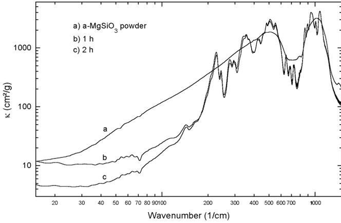
**Fig. 4.** Comparison of the IR spectrum of thermally untreated  $\text{MgSiO}_3$  glass powder (a) with the spectra of  $\text{MgSiO}_3$  glass powder that has been annealed at  $T=1121$  K for 1 and 2 h (b, c).
