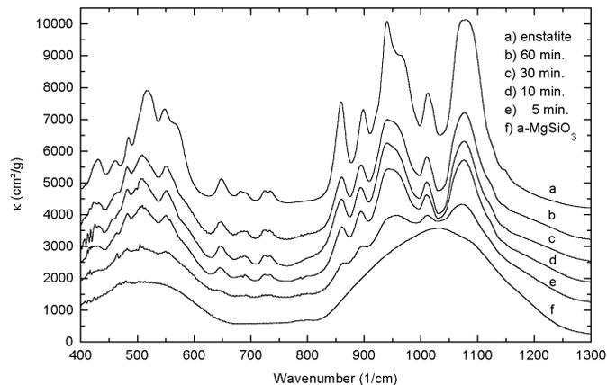
**Fig. 3.** Evolution of the MIR spectrum of  $\text{MgSiO}_3$  glass particles (f). At  $T=1121$  K, the annealing times for the spectra are indicated. For comparison, the enstatite spectrum (a, from Jäger et al. 1998) has been added. For clarity, the spectra are vertically shifted: a, b, c, d, e by +3500, +2500, +2000, +1500, +1000  $\text{cm}^2/\text{g}$ , respectively.
