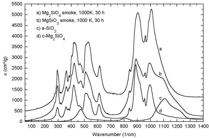
**Fig. 9.** The IR spectrum of annealed  $\text{Mg}_2\text{SiO}_4$  and  $\text{MgSiO}_3$  smoke (spectra a, b) compared with that of  $\text{a-SiO}_2$  (c) and  $\text{c-Mg}_2\text{SiO}_4$  (d) (Jäger et al. 1998). For clarity, spectra a is vertically shifted by  $+500 \text{ cm}^2/\text{g}$ . The spectra c and d are in arbitrary units.
