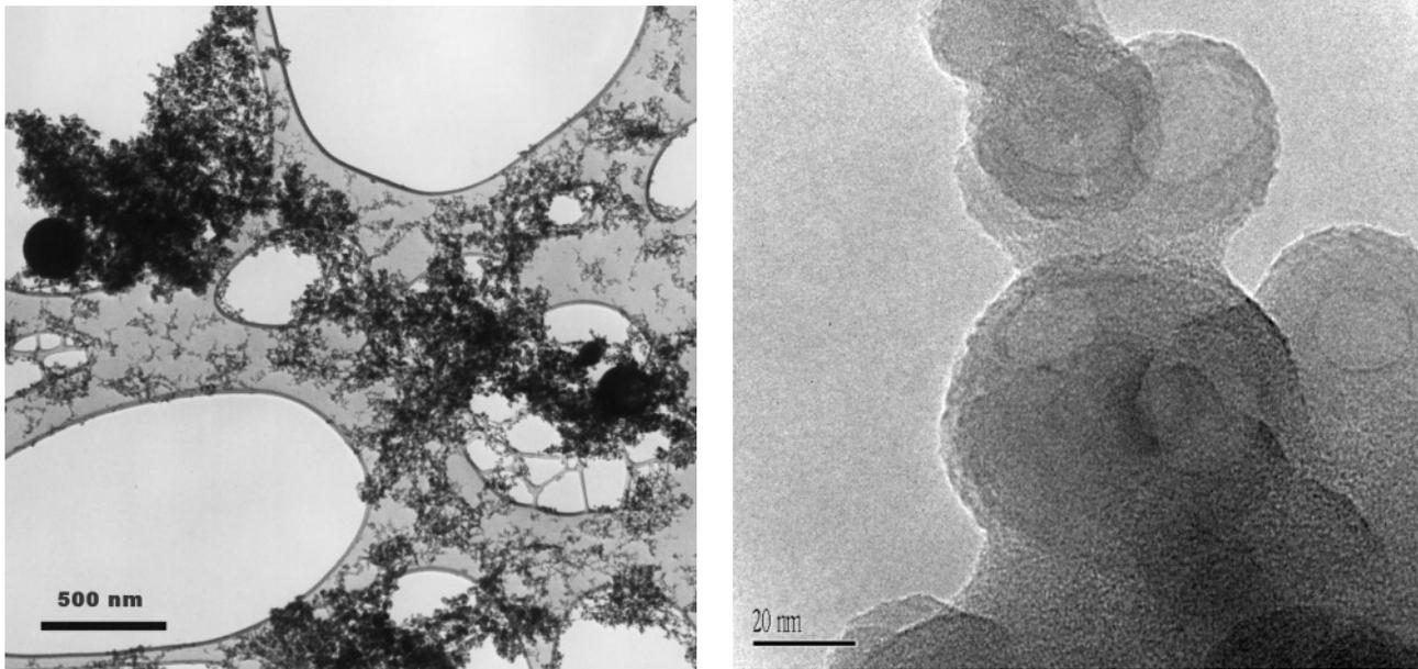
**Fig. 1.** TEM images of laser-ablated  $\text{MgSiO}_3$  smoke. Spherical micrometre- and nanometre-sized smoke particles are composed of nonstoichiometric Mg-silicates. In the particles with diameters ranging from 10 to 50 nm, voids are contained frequently.
