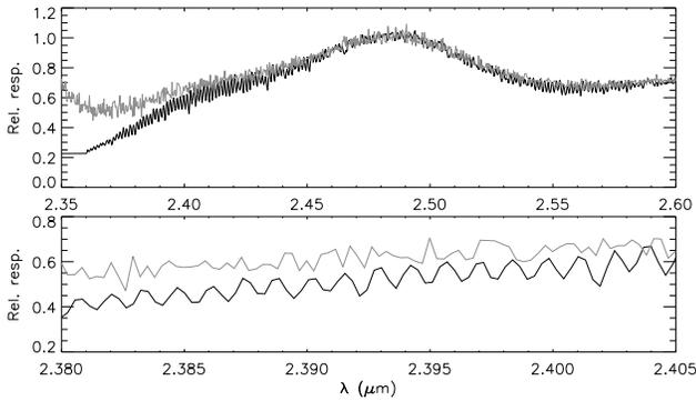
**Fig. 3.** The RSRF for AOT-band 1A derived from  $\alpha$  Lyr observations (black) *vs.* the RSRF as measured from an extended blackbody source in the laboratory (grey). The leakage is clearly visible in the laboratory measurement. As seen in the lower plot, only the in-orbit measurement (lower curve) fully resolves the fringes.
