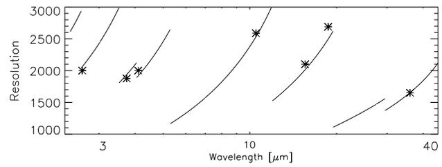
**Fig. 3.** The theoretical spectral resolution of both the SW and the LW section of the SWS, see text. The asterisks represent observed values from lines detected in the compact (nearly point source) Planetary Nebula IC 2501.
