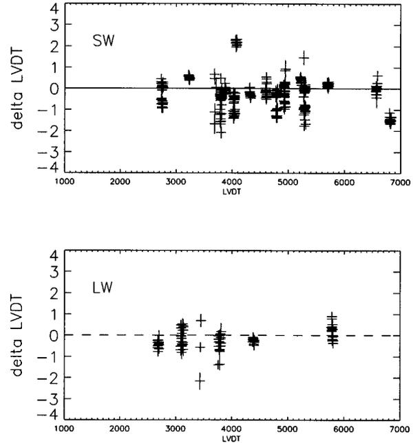
**Fig. 1.** Example residuals of the wavelength calibration in instrumental units LVDT from observations of Planetary Nebulae. Top figure: SW grating section using H recombination lines in NGC 7027, and ionic lines in IC 2501, Bottom figure: LW grating section, using ionic lines in IC 2501 (for wavelengths see Table 1).
