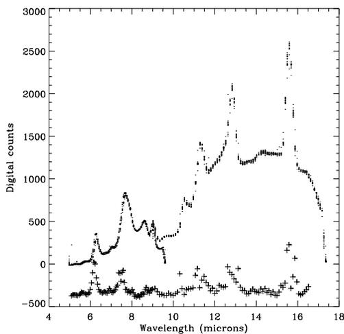
**Fig. 1.** Example of raw data (pixel [15,15] is illustrated here). Each measured datum is represented by a dot and there are 10 dots per scan leg; the vertical spread at each wavelength gives an idea of both the observation noise and of the reproducibility of the measurement on each leg of the CVF scan. The lower plot shows the RMS fluctuation of the averaged data. Note that the RMS plot has been magnified 10 times and shifted down by 400 units for clarity's sake.
