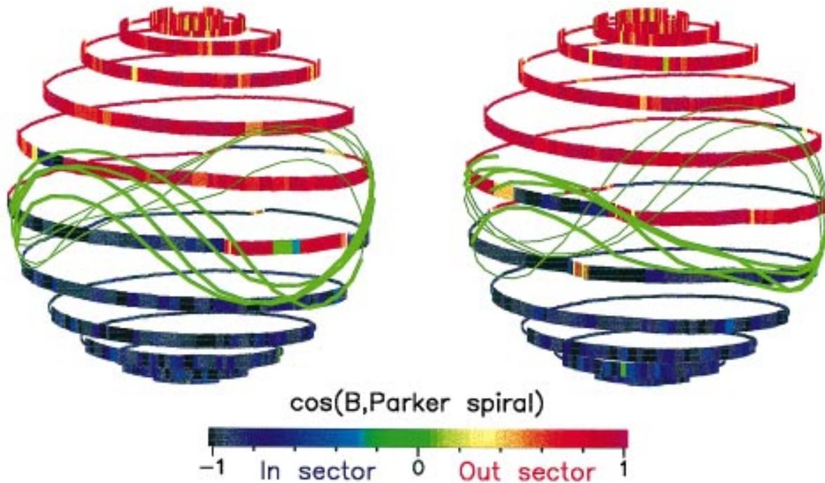
**Fig. 4.** A three dimensional representation of the polarity of the heliospheric magnetic field as observed by Ulysses, plotted using a colour scale based on the angle between the measured and expected field directions. Red represents antisunward polarities and blue sunward. The green lines show the location of the neutral line inferred from solar observations. The central meridian longitudes of the left and right panels are  $240^\circ$  and  $60^\circ$  respectively.
