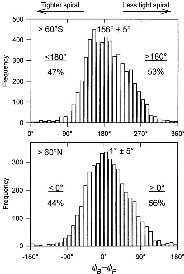
**Fig. 5.** Histograms of the deviations,  $\phi_B - \phi_P$ , of the azimuthal angle of the magnetic field from that predicted by the Parker model. The upper histogram is accumulated from data obtained at latitudes above  $60^\circ$  in the southern hemisphere and the lower histogram is the same for the northern hemisphere.
