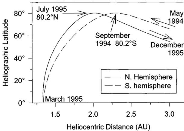
**Fig. 1.** The trajectory of Ulysses from May 1994 to December 1995. The absolute value of latitude is plotted against radial distance, thus emphasising the difference in the trajectory between the northern and southern hemispheres.
