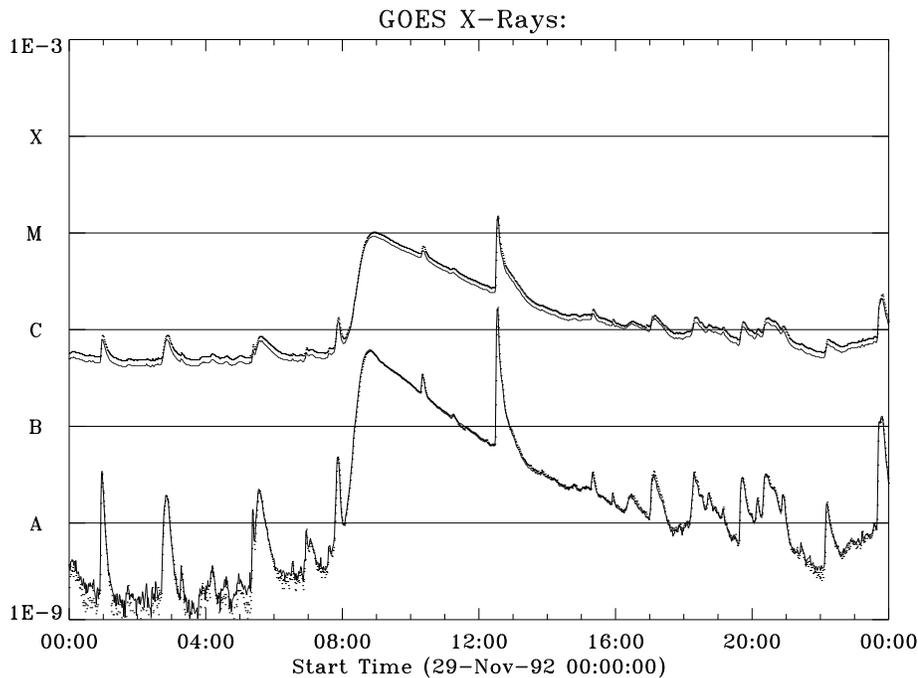
**Fig. 4.** Full-sun integrated x-ray fluxes ( $W/m^2$ ) measured by the GOES satellite on November 29, 1992. The upper traces are from the 1 - 8 Å wavelength band and the lower from the 0.5 - 4 Å band.
