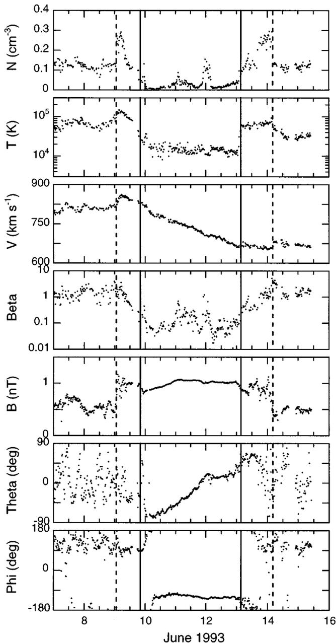
**Fig. 5.** Plasma and magnetic field parameters observed by Ulysses for the CME encountered between June 10-12, 1993. The format is the same as Fig. 2. The vertical dashed lines denote forward and reverse shocks driven by over-expansion of the CME.
