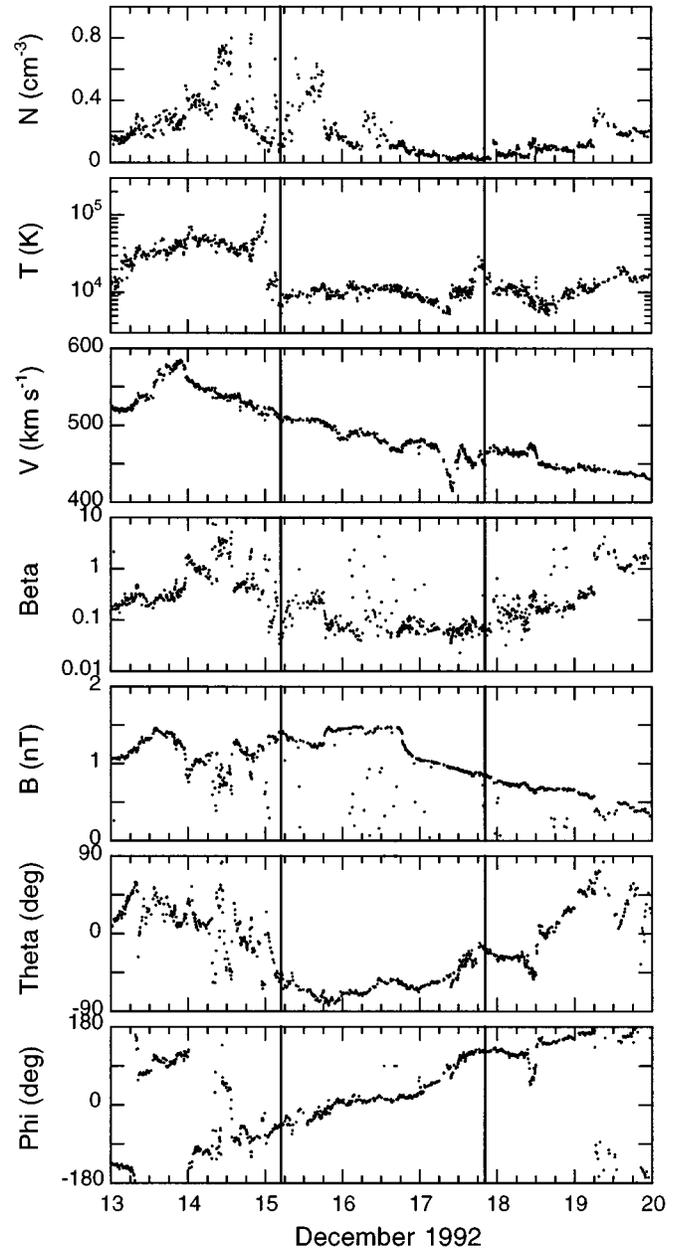
**Fig. 2.** Selected plasma and magnetic field parameters observed by Ulysses in association with the passage of an interplanetary CME between December 15–17, 1992. Plotted from top to bottom are proton density, proton temperature, bulk flow speed, total plasma beta, magnetic field magnitude, and polar and azimuthal angle of the magnetic field. The interval of bi-directional electron flux is marked with vertical lines.
