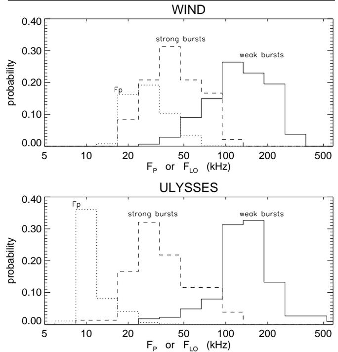
**Fig. 4.** Histograms of  $f_p$  and  $f_{lo}$  showing how the low frequency cutoffs are strongly affected by burst intensity but are essentially independent of the value of  $f_p$  at the spacecraft.
