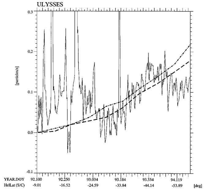
**Fig. 7a.** Counting rates of the background corrected and normalized ELH channels which are interpreted as being caused by protons with  $E > 230$  MeV, from 100/1992 to 185/1994 ( $-9^\circ$  to  $-55^\circ$  heliographic latitude), together with theoretical expectations (see text for details).
