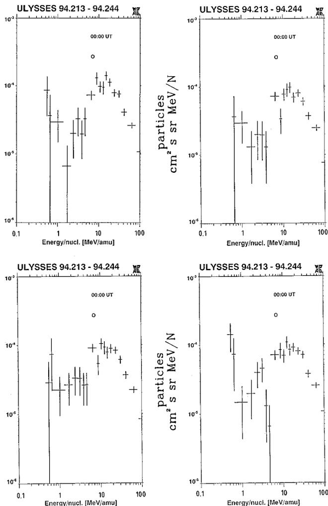
**Fig. 10.** Energy spectra of anomalous oxygen during quiet periods after switch off of the back detectors, shown for the 4 telescopes T1–T4. This extends the energy range normally covered by the instrument, shown in Fig. 8, to almost 100 MeV/N.
