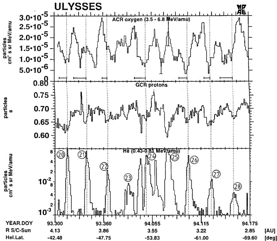
**Fig. 9.** Fluxes of anomalous oxygen (3.5 to 6.8 MeV/N, upper panel) together with GCR protons ( $E > 230$  MeV, mid panel) and helium (0.43 to 0.81 MeV/N, lower panel).
