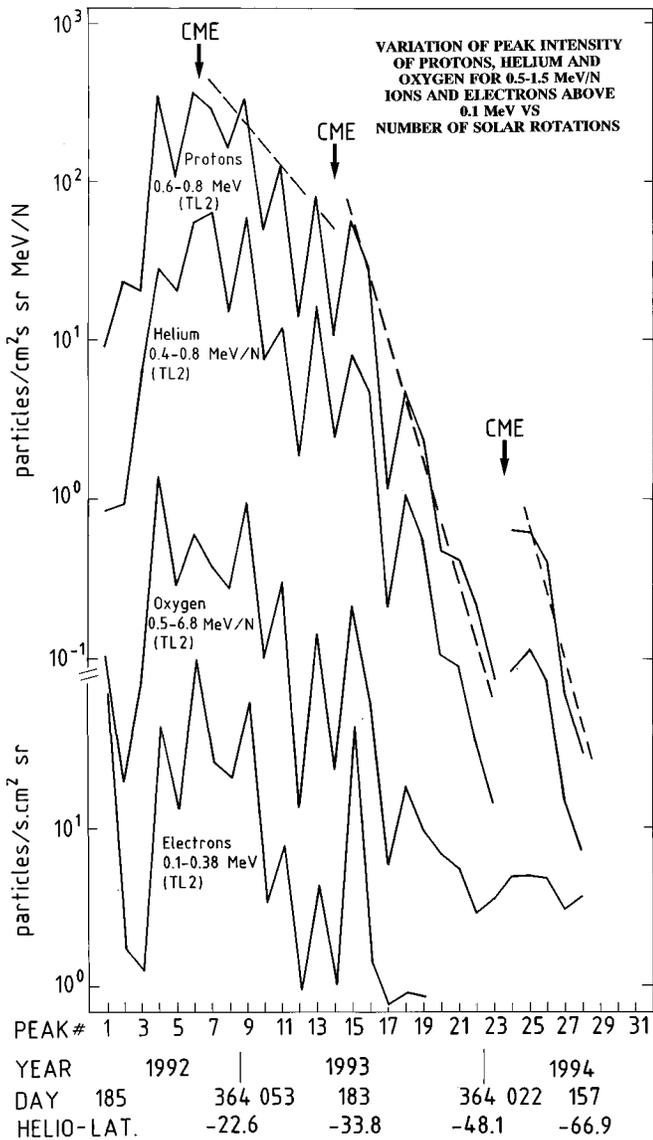
**Fig. 6.** Variations of observed peak intensities of protons, helium, oxygen and electrons during the high latitude path of ULYSSES. Abscissa is in solar rotations, numbers as in Fig. 1a.
