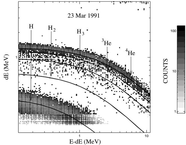
**Fig. 1.** Pulse height analysis histogram map of the energy loss in the thin forward detector vs the following detector. Plotted are the data for March 23, 1991, a period of high particle flux. Shown are the theoretical energy loss curves for some of the ion species detected with HI-SCALE (H, di-hydrogen, tri-hydrogen,  $^3\text{He}$ ,  $^4\text{He}$ ).
