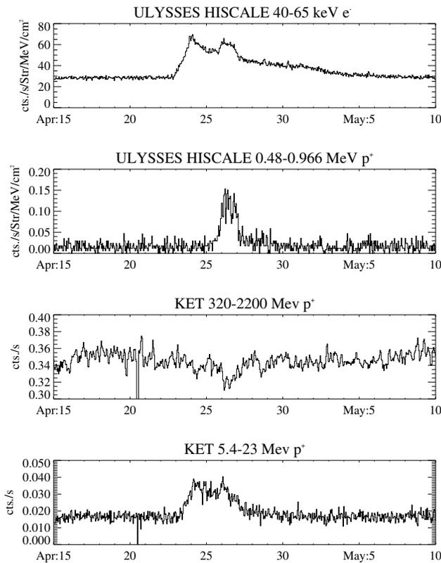
**Fig. 1.** Hourly averaged data from the Ulysses HI-SCALE and KET instruments are plotted here versus time from April 15 to May 05, 1995. From top to bottom the four panels display HI-SCALE 40–65 keV electron fluxes; HI-SCALE 0.480–0.966 keV proton fluxes; KET 320–2200 MeV protons counting rates and KET 5.4–23 MeV proton counting rates.
