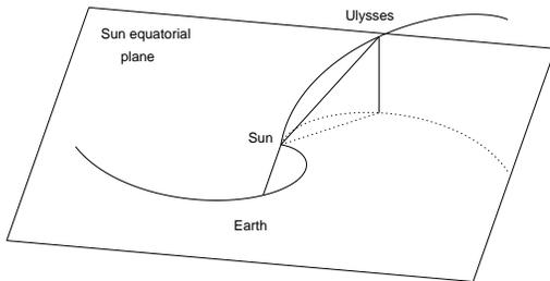
**Fig. 2.** Parker spiral geometry for April 22, 1995 for Ulysses spacecraft and WIND/Earth connections. The Ulysses spacecraft spiral has been computed for a solar wind speed of 750 km/s. WIND/Earth spiral has been computed for a solar wind speed of 310 km/s and is represented in dotted line. See Table 1 for details. The projections of the corresponding spirals onto the ecliptic are represented at the bottom of the figure.
