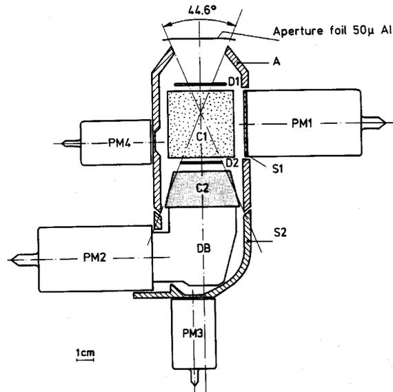
Fig. 1. Cross section of the KET instrument.
