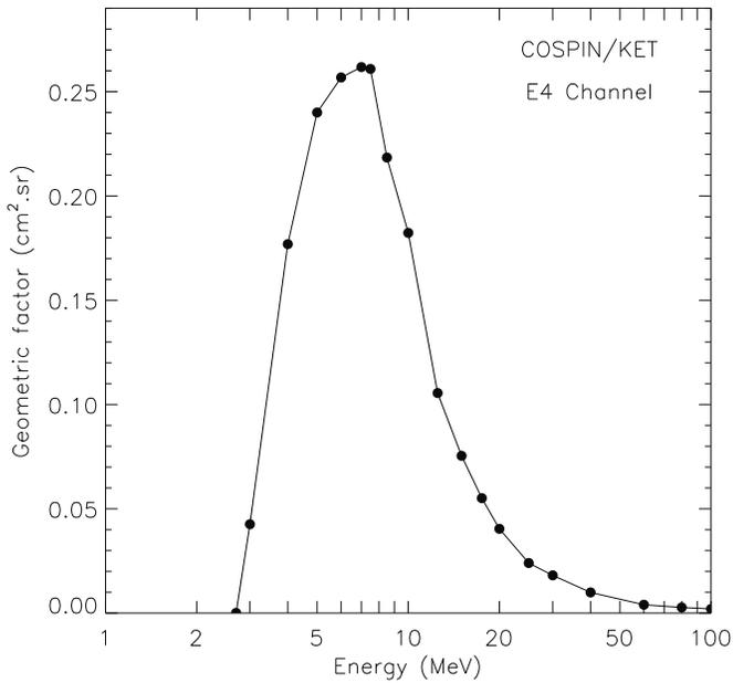
**Fig. 2.** Geometric factor of the E4 electron channel.
