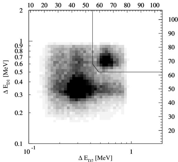
**Fig. 3.** D1-D2 PHA distribution for E4 events. The axis are labelled in channels and in the corresponding energy losses. The peaks are located at one and two times the signals for a singly charged minimum ionizing particle. The heavy line marks the selection chosen between E4<sub>1el</sub> and E4<sub>2el</sub> events.
