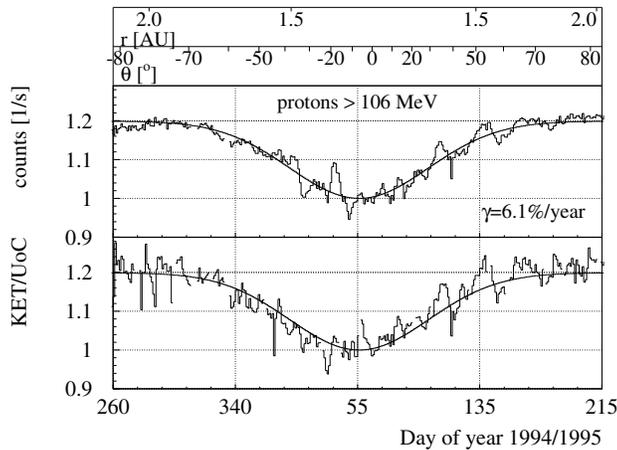
**Fig. 3.** Upper panel: temporally detrended daily averaged counting rate for  $>106$  MeV protons and approximation by Eq. 3. Lower panel: daily averaged counting rate ratio of  $>106$  MeV protons and same approximation as in the upper panel.
