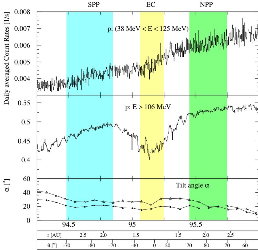
**Fig. 1.** Daily averaged counting rates from the KET instrument and 27-day averaged tilt angle for the northern (filled  $\triangle$ ) and southern (open  $\triangle$ ) hemisphere. S.P.P. = southern polar passage, N.P.P. = northern polar passage.
