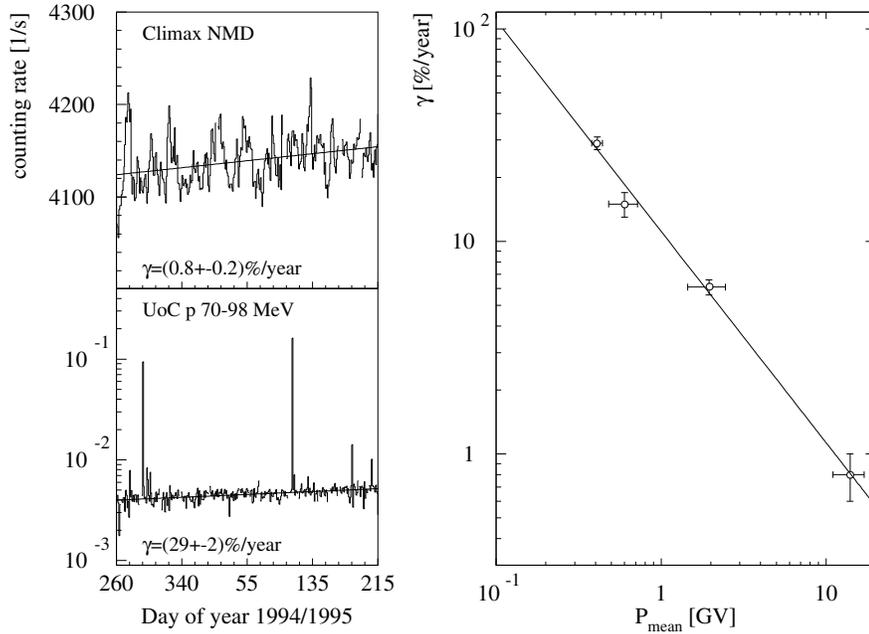
**Fig. 2.** Left: daily averaged counting rates measured by the UoC instrument on board IMP8 and UoC Climax neutron monitor and approximation by Eq. 1. Right: variation  $\gamma$  in %/year of daily averaged counting rates from the UoC instrument on IMP 8 and the UoC Climax neutron monitor.
