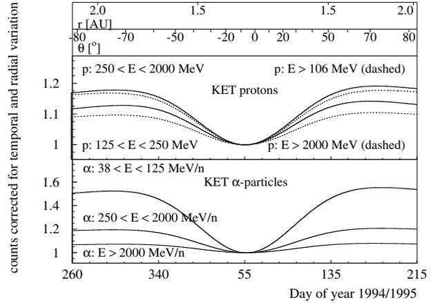
**Fig. 5.** Approximation (Eq. 3) for temporally detrended counting rates of protons (upper panel) and helium nuclei (lower panel) as a function of Ulysses heliographic latitude. The two lowest curves in the upper panel are for 125–250 MeV (solid line) and for  $>2000$  MeV protons (dashed line). Protons in the energy range of 250–2000 MeV have the largest polar flux excess.
