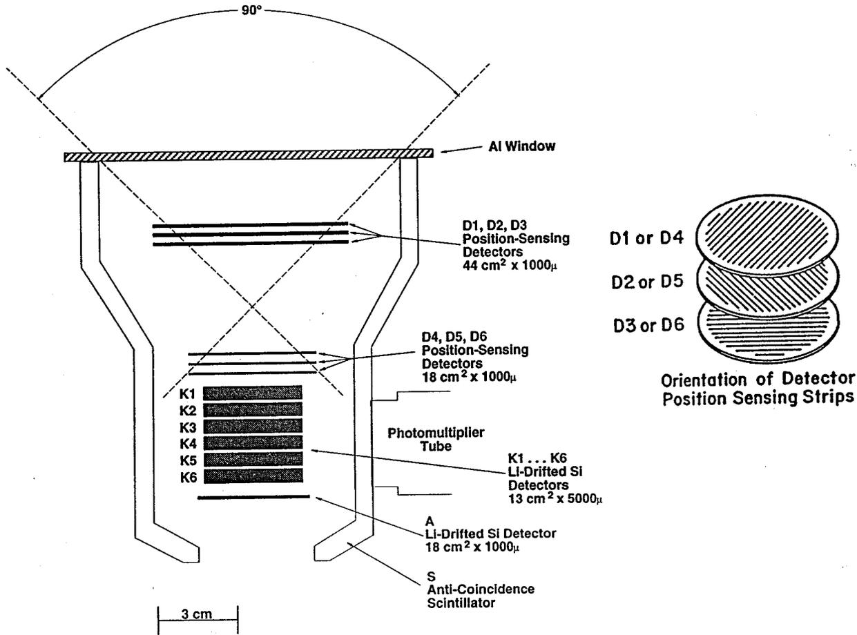
Fig. 1. a Cross section of Ulysses HET. b Position sensing silicon detector orientation (Simpson et al., 1992)
