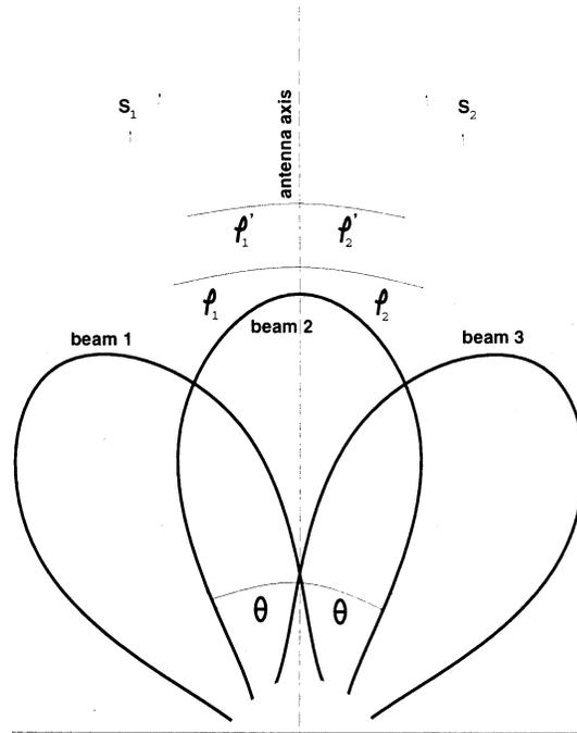
**Fig. 1.** Sketch of a simple antenna beam pattern of three intersecting beams observing two sources that emit at the same time.
