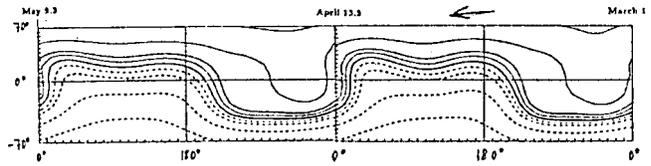
**Fig. 4.** Synoptic maps of the source surface magnetic field for the interval of the DIFOS records. Isolines correspond to 0, 1, 2, 5, 10, and 20  $\mu$ Tesla. Magnetic field data from the John Wilcox Observatory.
