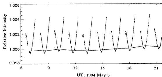
**Fig. 1.** Example of DIFOS raw data over 10 satellite orbits from the window 400–1000 nm. The curve connects mean values of each orbit.
