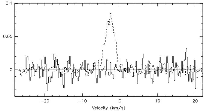
**Fig. 4.** DR21  $\text{C}^{18}\text{O}$  ( $J:2-1$ ) and  $^{16}\text{O}^{18}\text{O}$  ( $(N, J) = (2, 1) - (0, 1)$ ) spectra. The rms noise is 11 mK for 0.2 km/s resolution. The  $\text{C}^{18}\text{O}$  line has been divided by 40.
