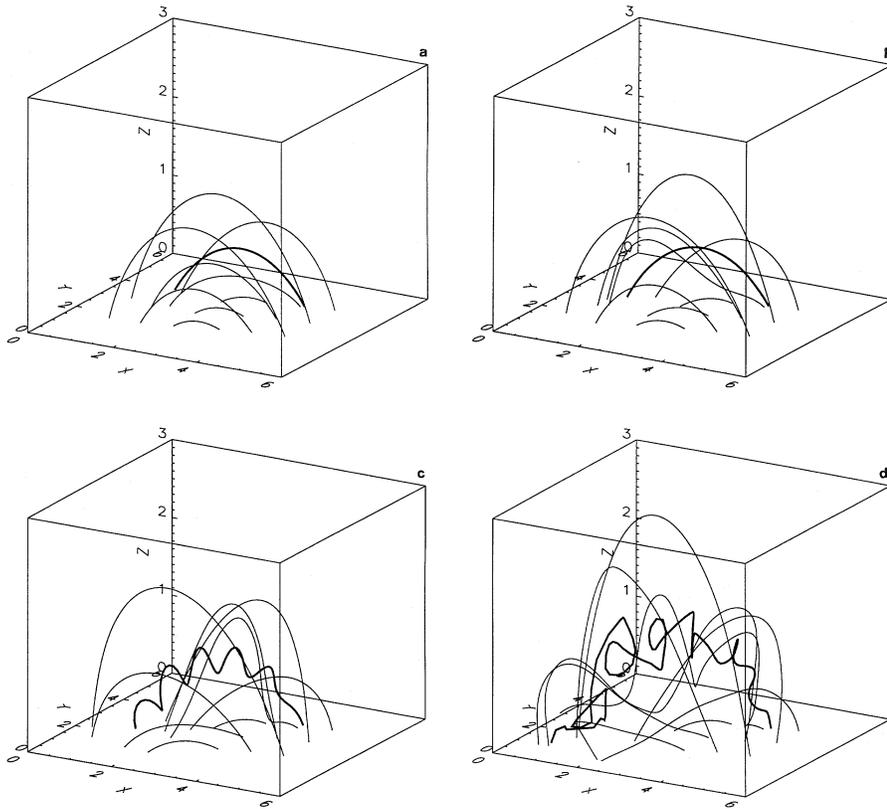
**Fig. 1a–d.** The single electric current path (thick line) and magnetic field (thin lines) for  $I = 5 \times 10^{10}$  A **a**,  $I = 1 \times 10^{11}$  A **b**,  $I = 2 \times 10^{11}$  A **c**, and  $3 \times 10^{11}$  A **d**. The distances are expressed in  $10^4$  km.
