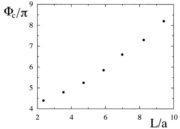
**Fig. 4.** The critical twist value  $\Phi_c$  as a function of the aspect ratio  $L/a$
