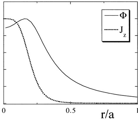
**Fig. 2.** The twist  $\Phi$  profile as a function of the normalized radius  $r/a$  (in arbitrary units), and  $J_z$  the resulting axial component of the current density
