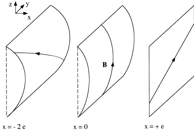
**Fig. 11a.** A simplified slab tied magnetic configuration in the vicinity of  $x = 0$
