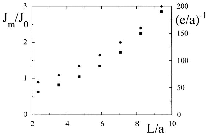
**Fig. 7.** The amplitude of the normalized current concentration (circles) and the normalized thickness of the current layer (squares) as a function of the aspect ratio  $L/a$ , measured at the axial midplane  $z = 0$
