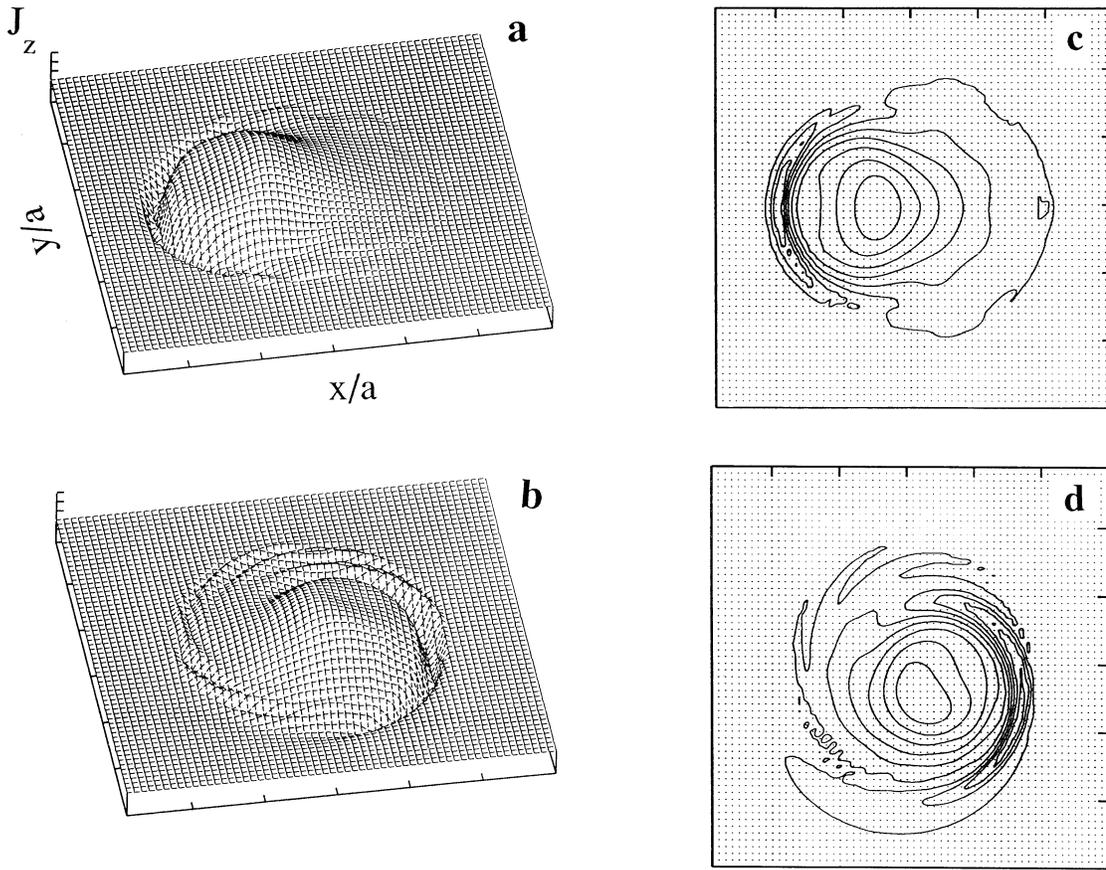
**Fig. 5a–d.** The axial component of the current density for the two axial planes: **a**  $z = 0$  and **b**  $z = L/4$ , and the corresponding iso-contours: **c** for  $z = 0$  and **d** for  $z = L/4$
