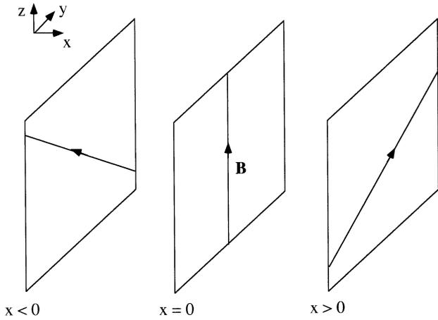
**Fig. 9a.** A simplified slab un-tied magnetic configuration in the vicinity of  $x = 0$
