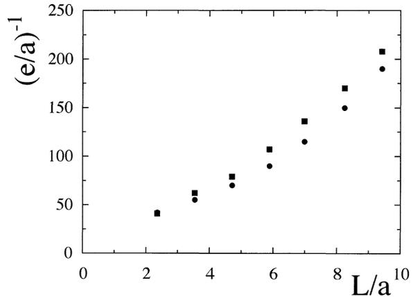
**Fig. 13.** The normalized thickness of the current layer at the axial midplane  $z = 0$ , measured in the simulations (circles), and calculated using Eq. 17 (squares) with  $C = 0.27a$  and  $A = 8$
