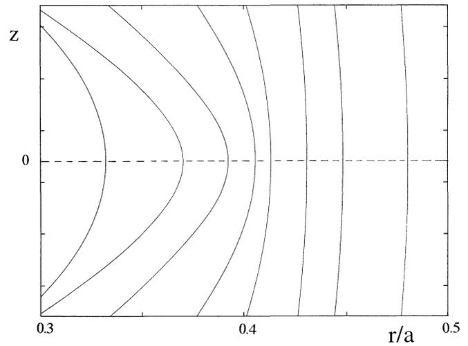
**Fig. 10.** The projections of different magnetic field lines in the  $(r, z)$  plane for an aspect ratio value  $L/a = 4.7$ , the  $z = 0$  axis is represented by the hatched line
