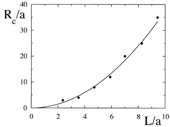
**Fig. 12.** The normalized curvature radius at  $x = 0$  at the axial midplane  $z = 0$  as a function of the aspect ratio value  $L/a$ , measured in the simulations (circles), and values obtained using Eq. (17) with  $C = 0.27a$  (plain line)
