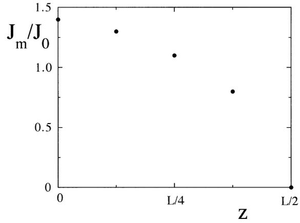
**Fig. 8.** The amplitude of the normalized current concentration as a function of the axial coordinate  $z$ , for the case  $L/a = 4.7$
