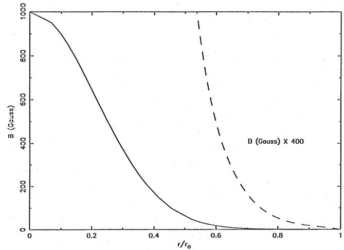
Fig. 1. Radial dependence of  $B_z$  the vertical component of the field
