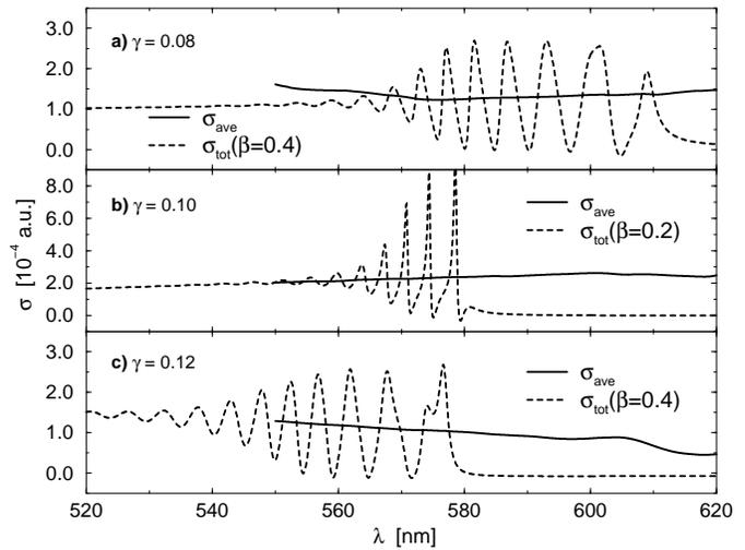
**Fig. 9.** Electric field averaged cross-sections  $\sigma_{ave}$  for  $\sigma^+$  polarization at magnetic fields  $\gamma = 0.08, 0.10, 0.12$  plotted together with a photoionization spectrum  $\sigma_{tot}$  at the same magnetic field and electric field  $F = \beta \cdot 10^7 V/m$ .
