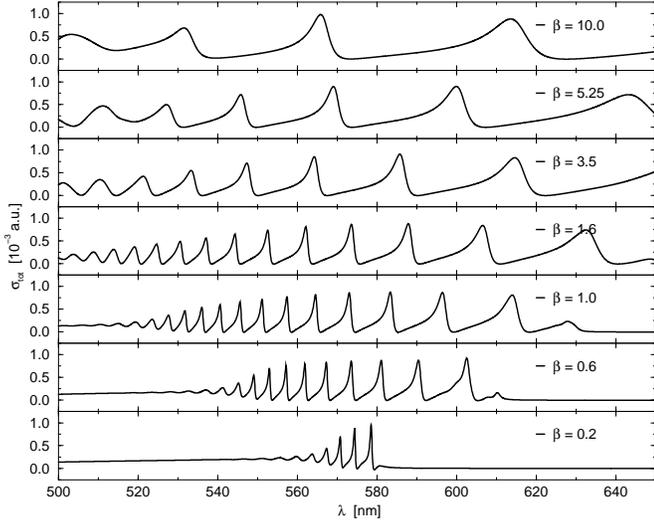
**Fig. 1.** Photoionization spectra in parallel fields for  $\sigma^+$  polarization from  $n = 3, m = -1$  initial states. The magnetic field is  $\gamma = 0.1$  for all spectra and the electric field is given by  $F = \beta \cdot F_H$  with  $F_H = 10^7$  V/m.
