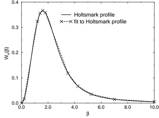
**Fig. 2.** The Holtzmark distribution of electric fields  $W_H(\beta)$ .  $\beta$  is defined by  $F/F_H$ , where  $F_H$  is the mean electric field. The Holtzmark profile is fitted by a choice of 11 points on the distribution and linear interpolation in between these points.
