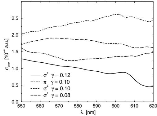
**Fig. 8.** Paschen opacities for the transitions of the previous figures averaged over a Holtsmark distribution of electric fields with  $F_H = 10^7$  V/m for wavelengths between 550 and 620 nm. Polarization and magnetic field as labeled,  $T = 15$  000 K.
