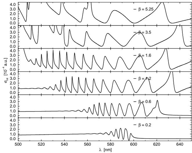
**Fig. 6.** Unnormalized Paschen opacities for  $\sigma^+$  transitions for magnetic field  $\gamma = 0.08$ , electric fields  $F = \beta \cdot 10^7$  V/m and temperature  $T = 15000$  K.
