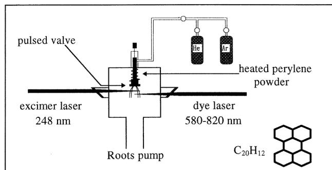
**Fig. 1.** A partial sketch of our experimental set-up. The pulsed jet supersonically expands into the vacuum chamber after mixing of the sample molecules with helium or argon carrier gas. It is first crossed with the excimer laser beam and, 1 cm downstream, with the dye laser one. The fluorescence signal induced by the dye laser is collected by a lens whose axis is perpendicular to the laser beams. It is then dispersed by monochromators and sent onto a photomultiplier or a CCD array.
