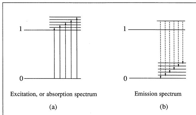
**Fig. 2a and b.** The meaning of LIF spectroscopy is outlined. **a** The excited state of the emitting species is probed when the total fluorescence signal (monochromator's slits widely opened) is sent to the photomultiplier (excitation, or absorption, spectrum). **b** Conversely, the species' ground state is probed while the fluorescence is dispersed in the monochromator (emission spectrum).
