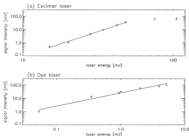
**Fig. 3a and b.** Relationships between the total fluorescence signal and **a** the excimer laser intensity, **b** the dye laser intensity at  $\lambda = 6290.7$  nm. The best fit lines have slopes of 3.96 and 0.89 respectively. Saturation can be seen in panel (a). Similar relationship was found for any resonant wavelength of the dye laser.
